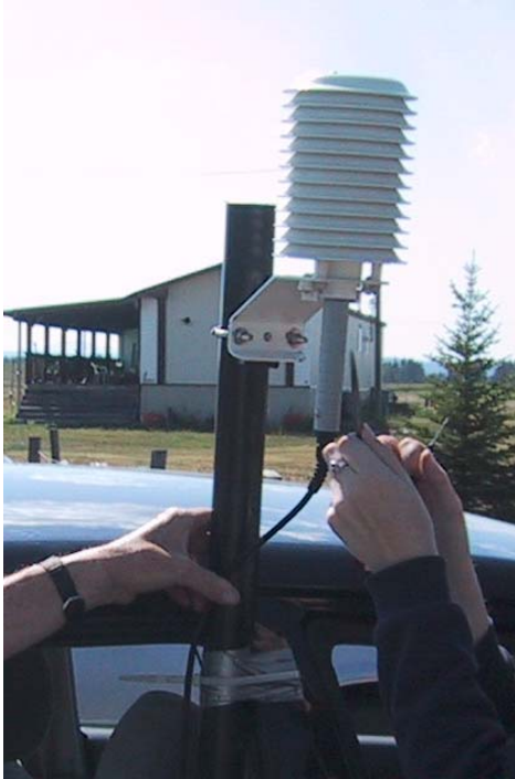
Figure 2.1. A temperature and relative humidity sensor mounted onto an economy-sized vehicle to perform mobile transects during the A-GAME field project in July 2003 (with a similar set-up for July 2004). The radiation shield containing the sensor was secured to a vertical length of PVC pipe above a rear window. For the July 2004 A-GAME field campaign, a pressure sensor was located on the back seat of the vehicle.
