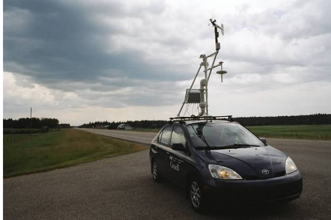
Figure 26: The Environment Canada Automated Mobile Meteorological Observation System (AMMOS), photo by Dave Sills.
