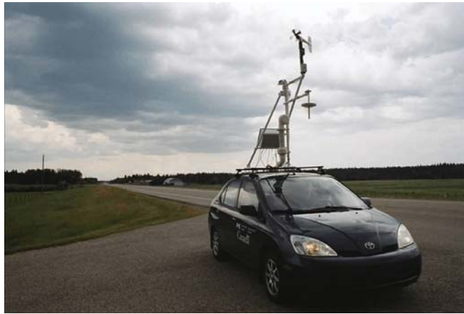
Figure 5: Environment Canada's Automated Mobile Meteorological Observation System (AMMOS), photo by David Sills.
