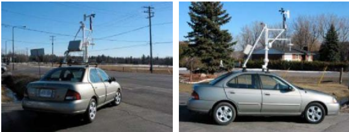
Figure 5: Mobile data collection platform purchased by the Cloud Physics and Severe Weather Research Section of Environment Canada. The equipment is designed to be mounted using a standard roof rack.
