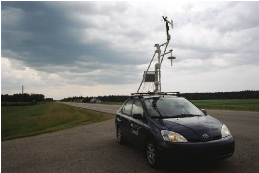
Figure 4: Photo by Sills of the mobile mesonet unit during testing on 23 July 2006.
