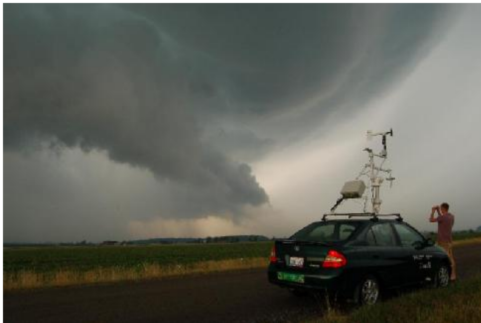
Figure 7: The Environment Canada Automated Mobile Meteorological Observation System (AMMOS). Photo by Dave Sills.
