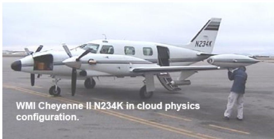
Figure 10: Instrumented Cheyenne II aircraft operated by WMI.
