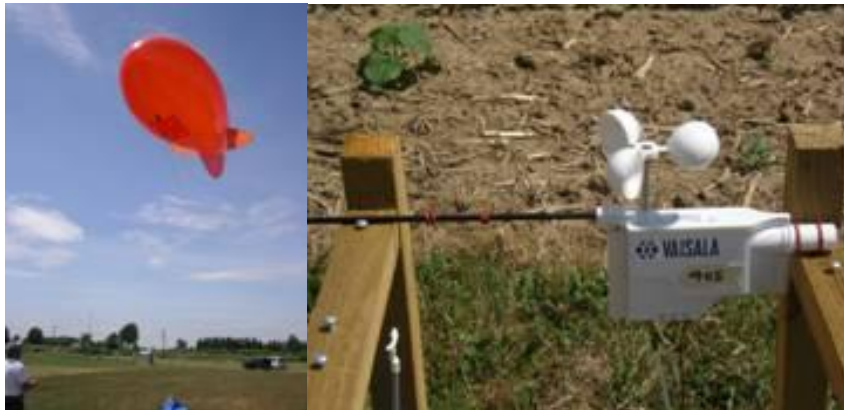
Figure 9: The Environment Canada tethersonde balloon (left) and close-up of a sonde.
