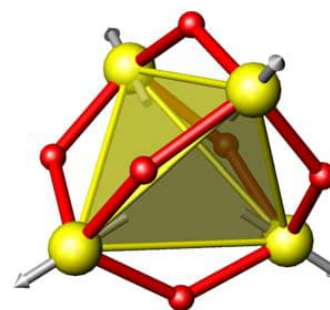
Figure 2: Tetrahedral spin arrangement on metals (yellow) with oxide (red) bridges responsible for magnetic exchange.
