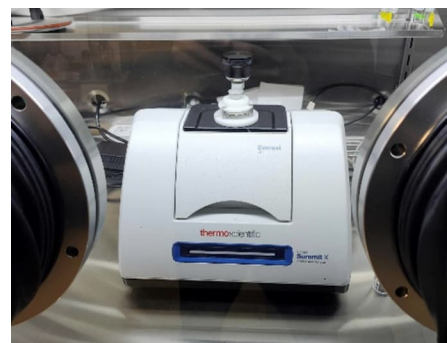
Figure 1 Recently installed FTIR spectrometer and operando electrochemical cell within Argon glovebox, waiting to be used.
